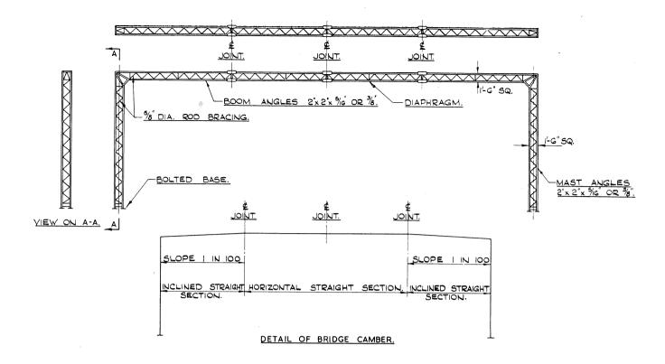
Fig.1 (a) Five track supporting structure (Max. span 75 ft.)
