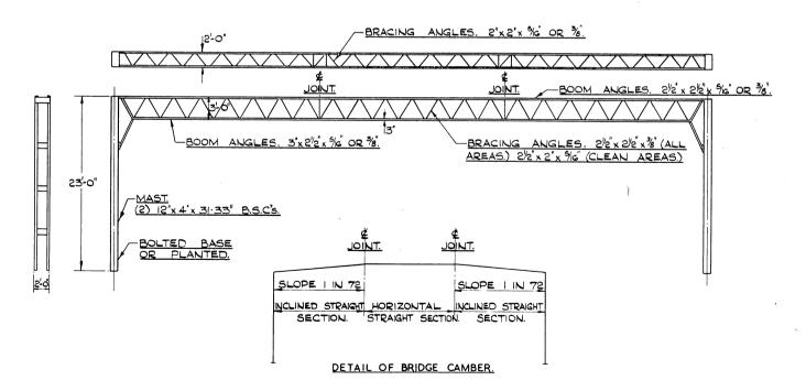
Fig.1 (b) Eight track supporting structure (Max. span 100 ft.)
