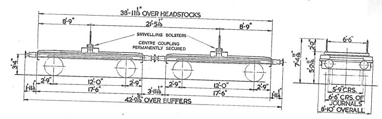
TARE: 19TONS 14CWTS MIN CURVE: 12 CHAINS
