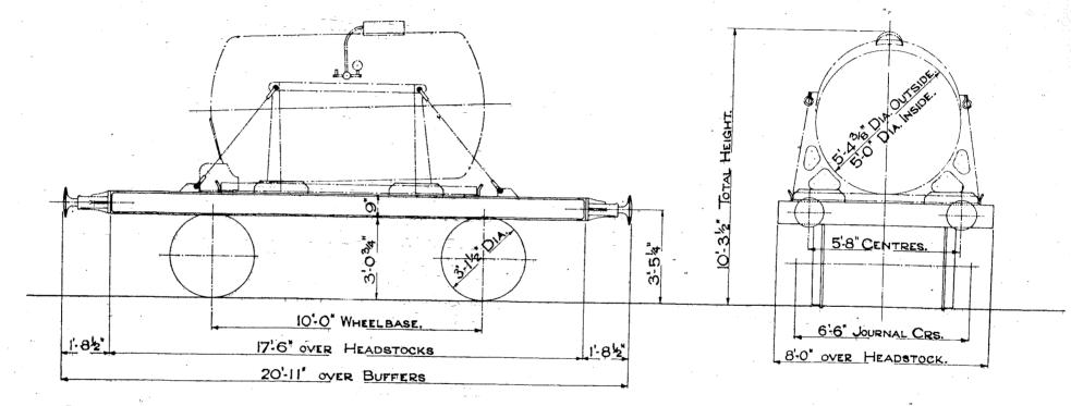
CODE TARE 5 TONS 11 CWTS. 7 TONS WITH TANK, CAPACITY OF TANK, 1080 GALLS.
