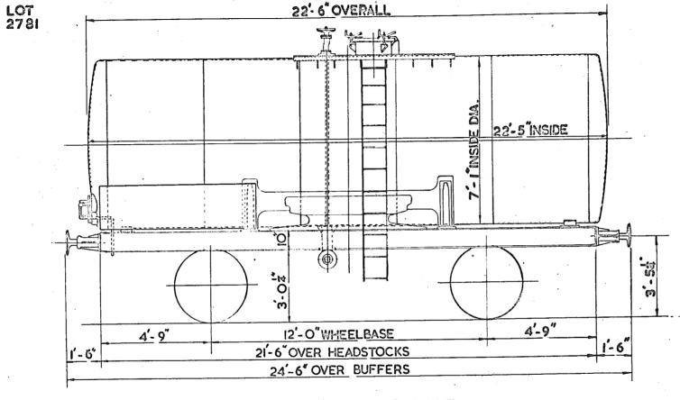
TARE 12 TONS 5 CWT. TEL. CODE CAPACITY - 5415 GALLONS (GROSS) BRAKE-STD. 20 TON HAND LEVER MINIMUM CURVE-IA CHAINS
