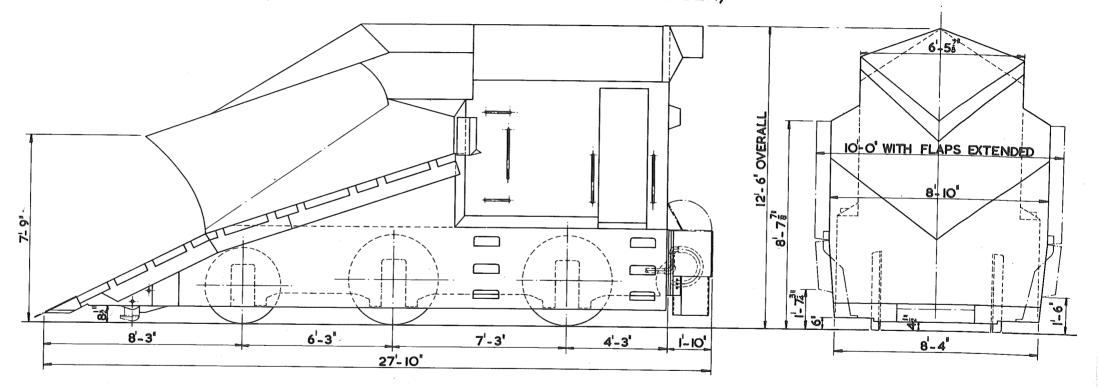
MINIMUM CURVE CHAIN TARE: 31 TON IOC.W.T. 3 QR.
