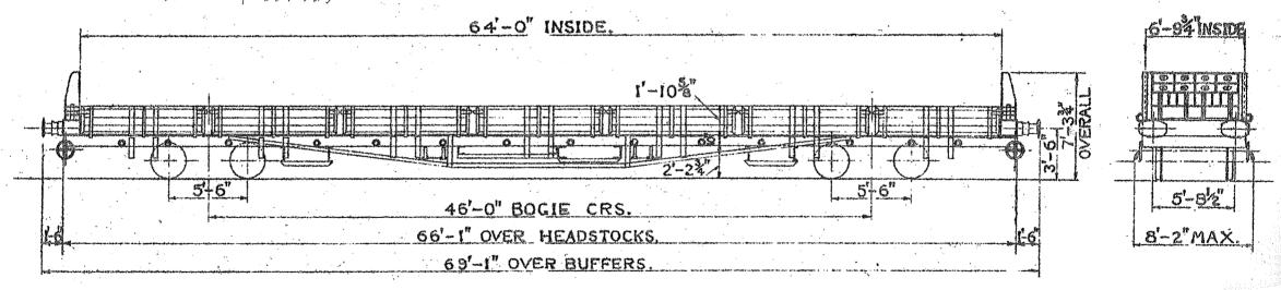
TEL. CODE STURGEON 'A'. TARE-27 TONS 18 CWT. MIN. CURVE 2 CHAINS. DOORS - 14 SIDE. BRAKE - SCREW HAND WHEEL. FLOOR AREA 436 SO.FT. BODY ENDS-STEEL.
