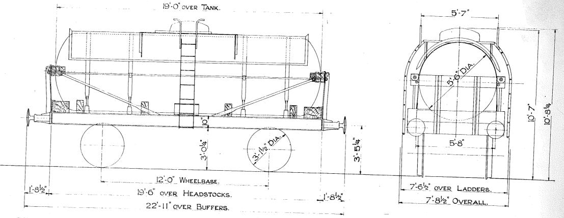
TEL. CODE. TARE 12 TONS 9 CWTS. CAPACITY OF TANK 2490 GALLS. STD. 20 TON LEVER BRAKE. THRO' PIPE. MINIMUM CURVE 1 4 CHAINS.
