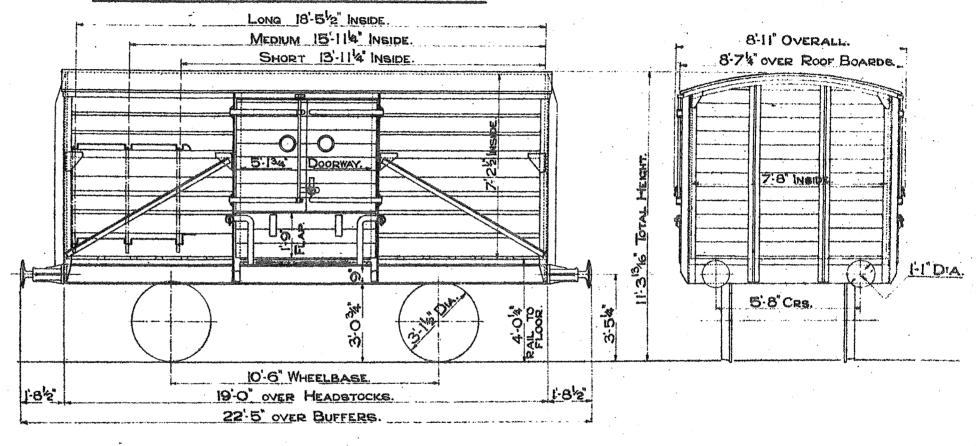
TEL. CODE-OXFIT. TARE 8 TONS 8 CWTS. FITTED A.V.B. & HAND LEVER. MINIMUM CURVE I CHAIN.
