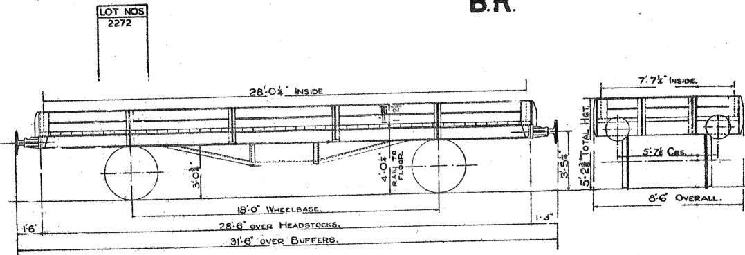
MIN. CURVE .: 2 CHAINS TARE :- 7 TON - 10 CWT. TEL. CODE :- WHITING. FLOOR AREA: 213 SQ. FT. CUBIC. CAP: 249CU. FT. CARRYING CAPACITY: 14 TON. FLOOR-WOOD. BRAKE - 20TON STD. HAND LEVER. BODY-WOOD.
