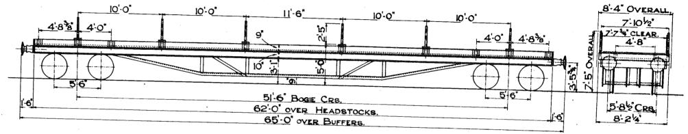
TEL.CODE-OYSTER GANE, A. TARE 21 TONS 12 CWTS. CARRYING CAPACITY 40 TONS. MINIMUM CURVE 2 CHAINS. ALL WOOD FLOOR. QUANTITY 104 NUMBERS - DB 996700 TO DB 996803.
