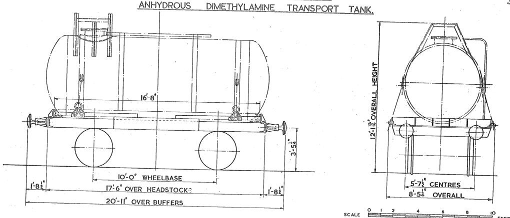
TARE IO TONS B CWTS. WITH TANK.
