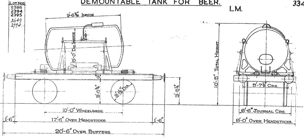
TARE WITH TANK 7TON-5CWT WITHOUT TANK 5TON-1 TEL. CODE-DOORS - NIL. BRAKE - AVB. & MORTON. CUBIC CAPACITY- 1080 GALLS. MINIMUM CURVE - I CHAIN.
