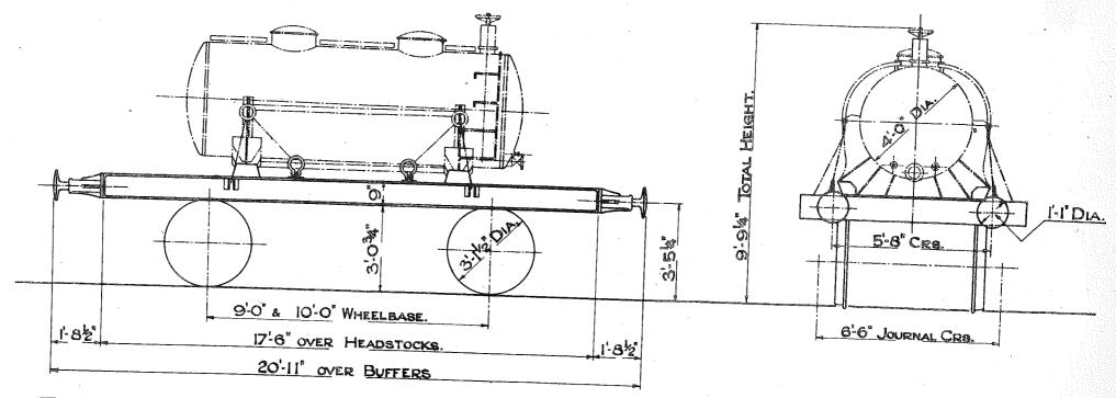
TEL. CODE TARE 6 TONS 15 CWTS. (WITH TANK.). 5 TONS 9 CWTS (WITHOUT TANK)
