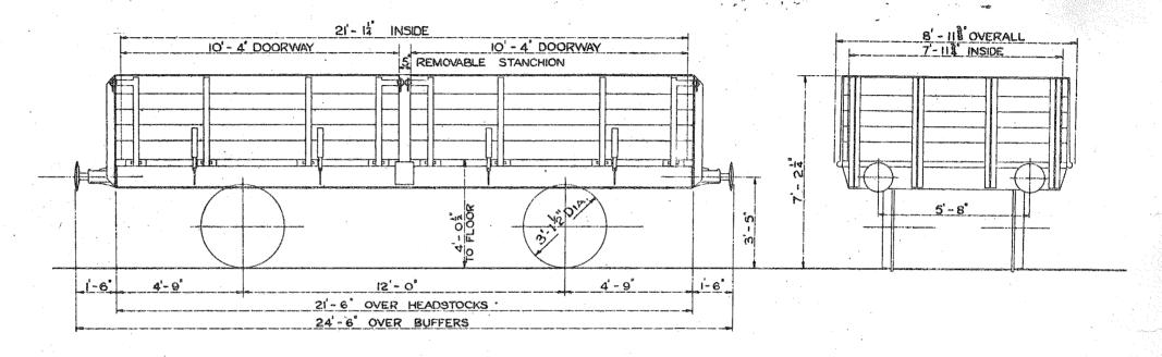
Tel. Code, PIPE Carrying Capacity, 12 tons. Type Of Brake, Std. 20 ton. Tare, 7 Tons 17 Cwts to 8 Tons 10 Cwts. Minimum Curve 14 Chains.
