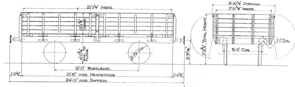
Tel. Code- Pipefit. Tare 8 Tons 12 Cwts. Capacity 530 Cu.Ft.
