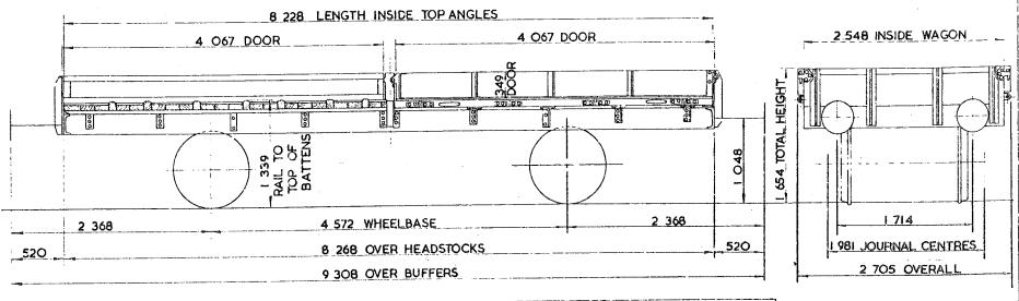
TARE IO 300 kg CARRYING CAPACITY - 22 500 kg CAPACITY - 6.861 m<sup>3</sup> MAX SPEED 50 mile/h WHEELS 952 DIA. JOURNALS - 124 DIA ROLLER BEARINGS
