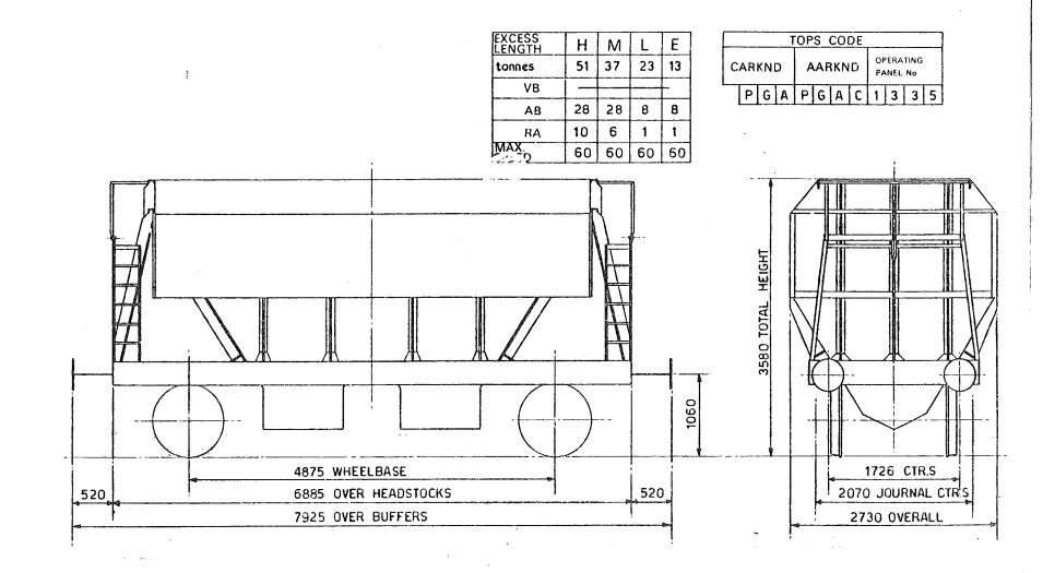
TARE - 12450kg CARRYING CAPACITY - 38500 kg CAPACITY - 28317 m<sup>3</sup> MAX. SPEED - 60 mile/h WHEELS - 952 DIA. JOURNALS - 150 ROLLER BEARING
