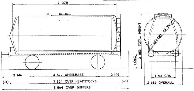
TARE \_ 14100 kg CARRYING CAPACITY- 31900 kg CAPACITY- 36118 litres. MAX SPEED - 60 mile/h WHEELS - 952 DIA. JOURNALS - 140 DIA. ROLLER BEARINGS BUFFERS-HYDRAULIC 406 DIA. HEADS. COUPLINGS - INSTANTER MIN. CURVE - 31 m GEN. ARRGT. DRG. No. --BRAKE-AIR BLOCK, VACUUM PIPED & HAND LEVER. SUSPENSION - FAT 26
