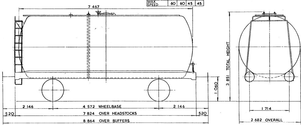
TARE - 14 750 kg CARRYING CAPACITY- 31 200 kg CAPACITY -38 822 litres MAX. SPEED - 60 mile/h WHEELS- 952 DIA. JOURNALS - 140 DIA, ROLLER BEARINGS BUFFERS-HYDRAULIC 406 DIA, HEADS COUPLINGS - INSTANTER MIN. CURVE - 31m GEN. ARRGT. DRG. No. -BRAKE- VACUUM BLOCK & HAND LEVER SUSPENSION - DOUBLE LINK
