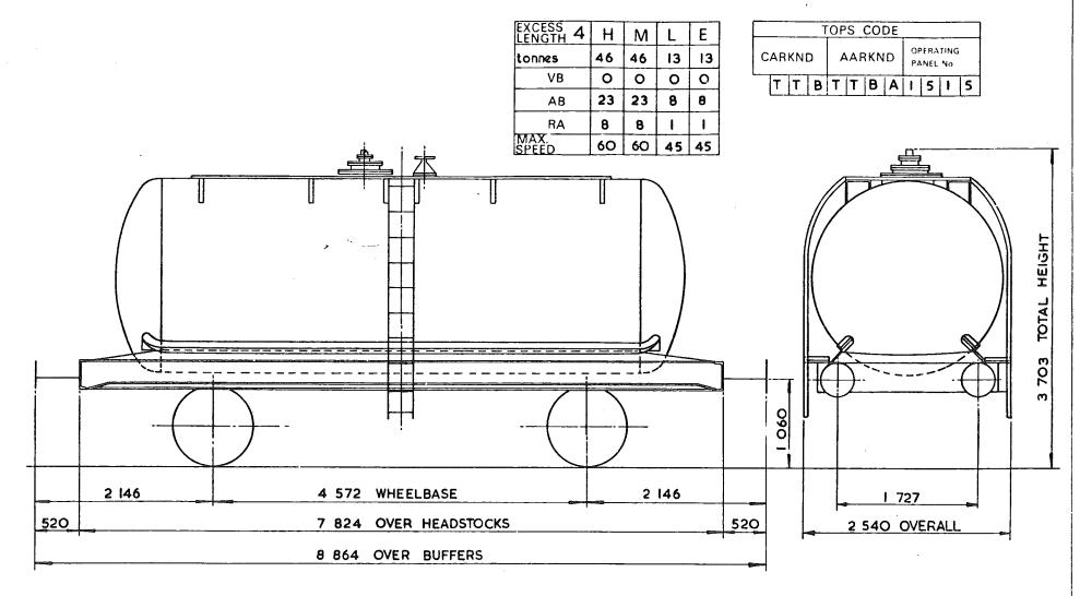
TARE - 12 950 kg CARRYING CAPACITY - 33 000 kg CAPACITY- 26730 litres MAX. SPEED - 60 mile/h WHEELS- 952 DIA. JOURNALS - 140 DIA. ROLLER BEARINGS
