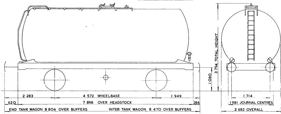
TARE - 16 950 kg CARRYING CAPACITY - 29000kg CAPACITY -32722 litres. MAX. SPEED - 60 mile/h WHEELS - 952 DIA. JOURNALS-140 DIA. ROLLER BEARINGS BUFFERS - HYDR AULIC 406 DIA. HEADS. COUPLINGS INTERNATIONAL SCREW, CLOSE COUPLED. MIN CURVE - 31 m GEN ARRGT DRG No. --BRAKE - AIR BLOCK, VACUUM PIPED & HAND LEVER . SUSPENSION - DOUBLE LINK
