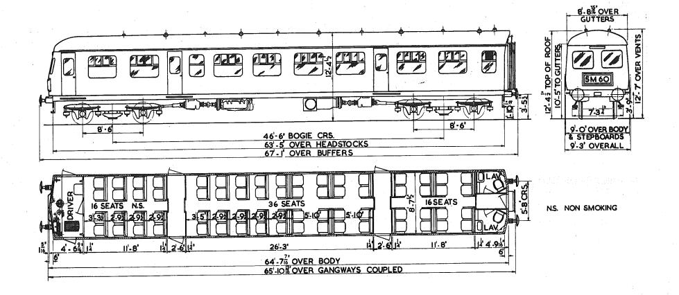
SEATS 66 TOILETS 2 COMPARTMENTS -GUARDS COMPARTMENTS -VENTILATION -CATERING EQUIPMENT - ORIGINAL DIAGRAMS FOR REFERENCE. - BR 637
