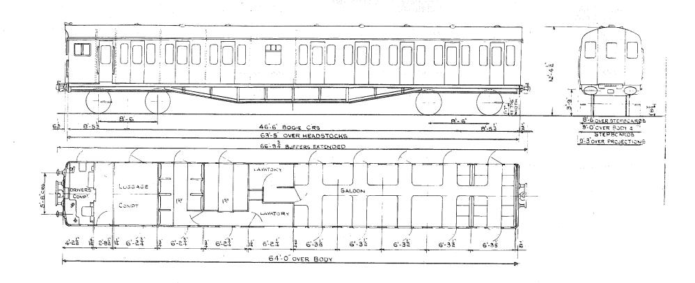
SEATS TOILETS COMPARTMENTS GUARDS COMPARTMENTS VENTILATION CATERING EQUIPMENT 13 FIRST CLASS 50 SECOND CLASS
