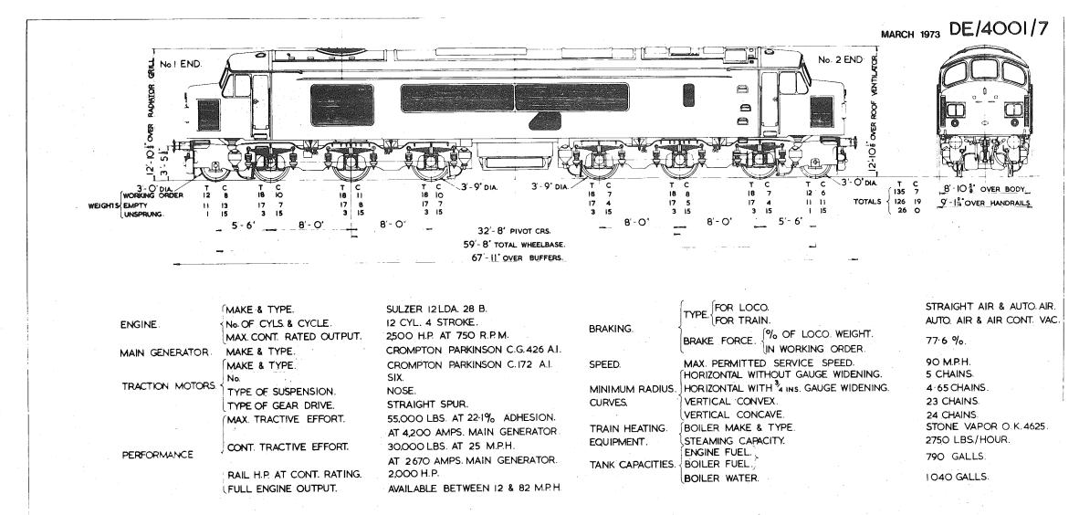
2500 H.P. B.R. TYPE 4 IC-CI DIESEL ELECTRIC LOCOMOTIVE. CLASS 45
