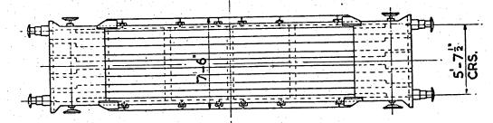
TARE: IN TON IOCWTS WITH BAULKS TARE: IO TON 9 CWTS WITHOUT BAULKS BRAKE: SCREW HAND & A.V. PIPE MIN. CURVE: 2 CHAINS FLOOR: WOOD & STEEL WHEELS:- 2'-8' DIA. JOURNALS:-9'×5" DIA. BUFFERS:- SELF CONTAINED BUFFER HEADS:-1'-1' DIA. COUPLINGS:-INSTANTER
