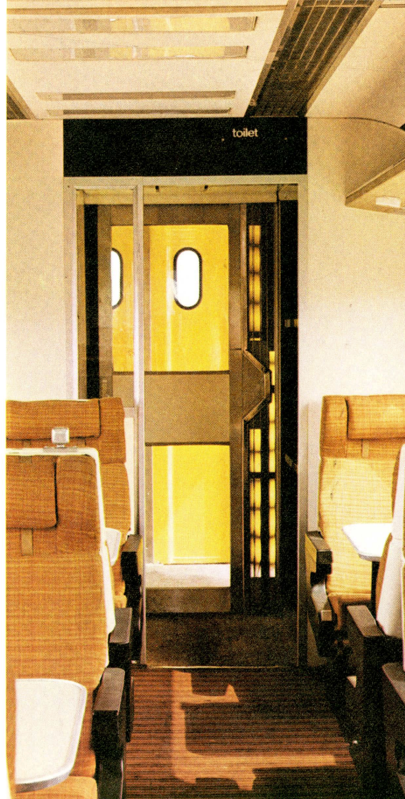
Interior doors operated automatically by tread-mats will help passengers with luggage to move easily along the train.
