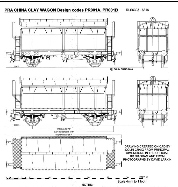
Built in 1983 by Standard Wagon Ltd., Heywood, and Reddish for Railease Ltd., using the chassis from redundant APCM pallet vans originally built in 1964 to Dia. 6/492.
