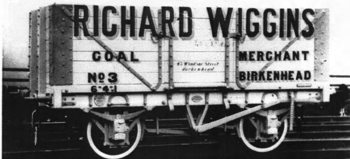
10-ton 7-plank coal wagon built by Hurst Nelson, probably some time around the turn of the century. Address on door is '43 Windsor Street/Birkenhead'. (HMRS photo no.ABN 329)
