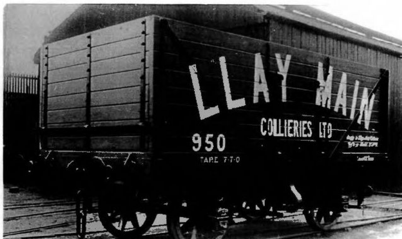
End-door 12-ton coal wagon built for Llay Main colliery; see pages 15/23 of this issue. This was the work-place of a neighbour when the Editor lived in East Saltney in the 1940s/1950s.
