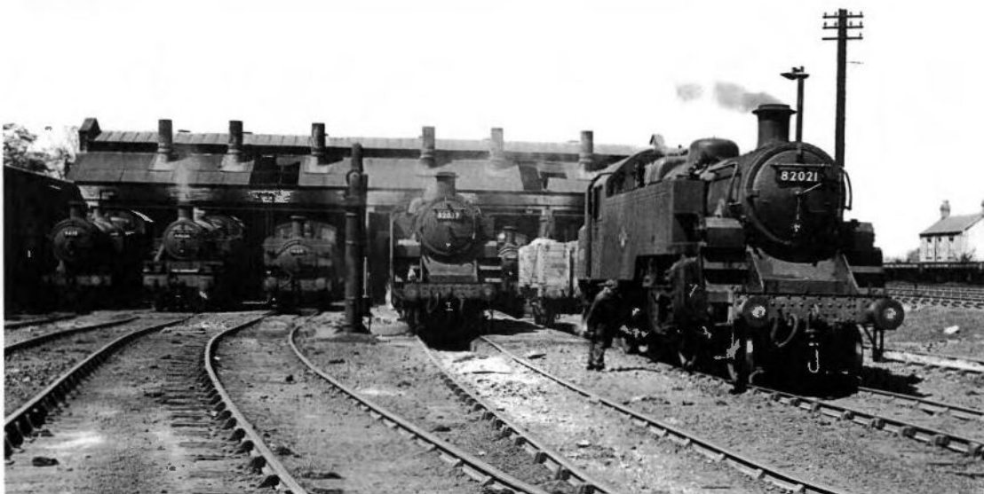
Rhosddu shed, Wrexham, photographed by Syd Wainwright on 21 June 1959. Left to right: 6610 (ex-GW 0-6-2T of 5600 class), 40126 (ex-LMS 2-6-2T of 3P class), 1669 (ex-GW pannier tank), 82037 (BR Standard), 1618 (ex-GW pannier), 82021 (BR standard).
