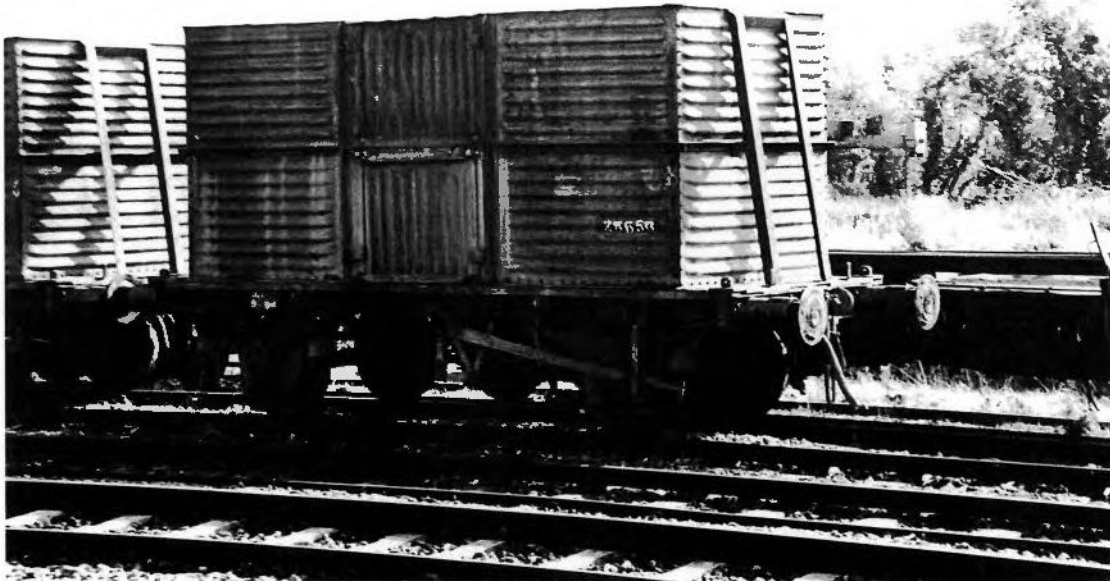
A later type of beet wagon: 28650 was photographed at Limerick Junction on 24 September 2004. It was one of a batch (nos.28501-28665) which were a combination of the underframes of redundant 4-wheel container flat wagons (from nos.25436-25983) with the sides and ends of two scrapped open wagons welded on top. These conversions dated from 1985 and were mostly used between a concentration depot at Wellington Bridge and the Thurles sugar factory. Waste not, want not!
