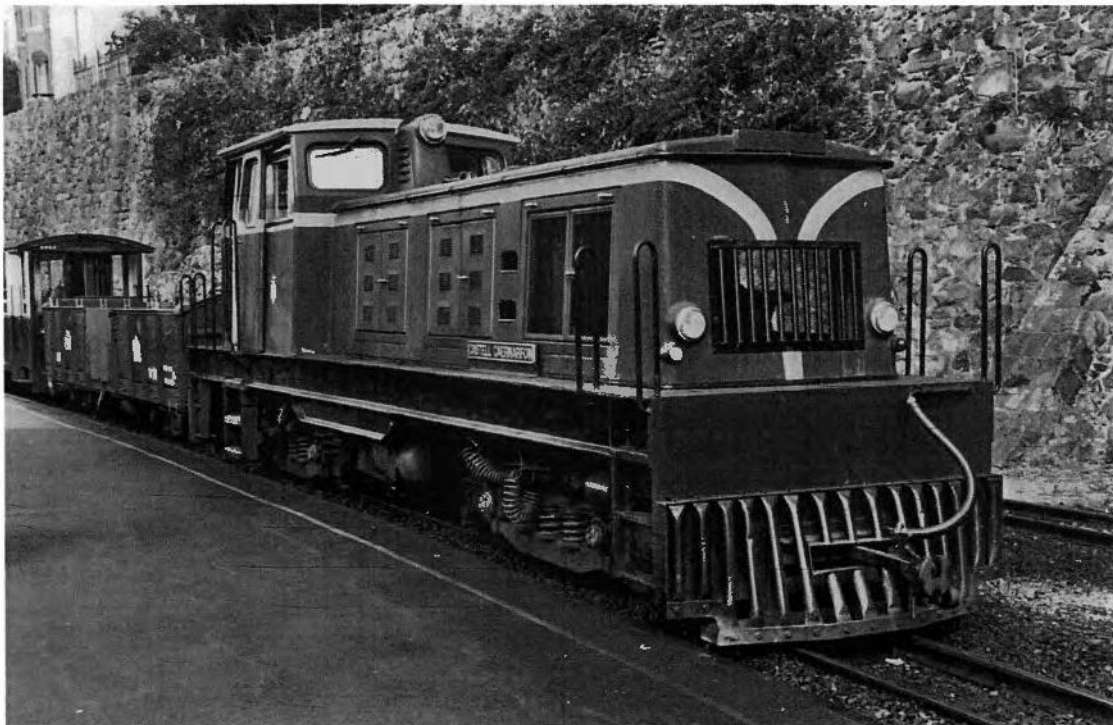
A different sort of oil-fired locomotive – 'Castell Caernarfon' at the Caernarfon terminus on 13 September 2008. This is a 335h.p. diesel hydraulic locomotive, originally built for a South African diamond mine in 1967. Came to Dinas in 1997 and re-bodied for the W.H.R. loading gauge
