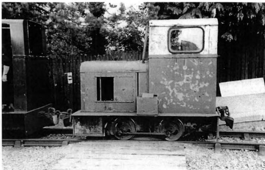
LM 259 (Deutz KS28B class 0-4-0DM, built 1965; 28hp, 3.4tons, 4-speed mechanical, 1ft 4½ins wheel diameter. Originally allocated to Boora bog in Co. Offaly). Photographed on 11 June 2004 at Kilmadan. Typical small Bord na Mona diesel – more recent engines are much larger.
