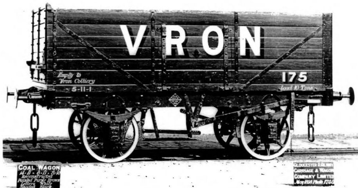
A 10-ton private owner coal wagon operated by Vron Colliery, which was just south of Brymbo near Wrexham. This 6-plank end door wagon had just been rebuilt by the Gloucester Railway Carriage & Wagon Co. in 1898, presumably from dumb-buffered form; it was painted purple/brown with black ironwork and black-shaded white lettering. (HMRS photo).
