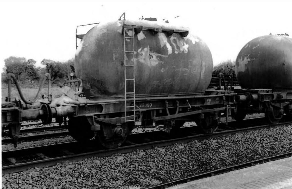
25097 from the third batch (1967): no lifting lugs on solebar, smaller buffer guides, rectangular cover for unloading manifold. The paler patches on the tank are where caked cement dust has come off – in a different pattern on every wagon! Photographed at Limerick Junction on 27 May 2003.
