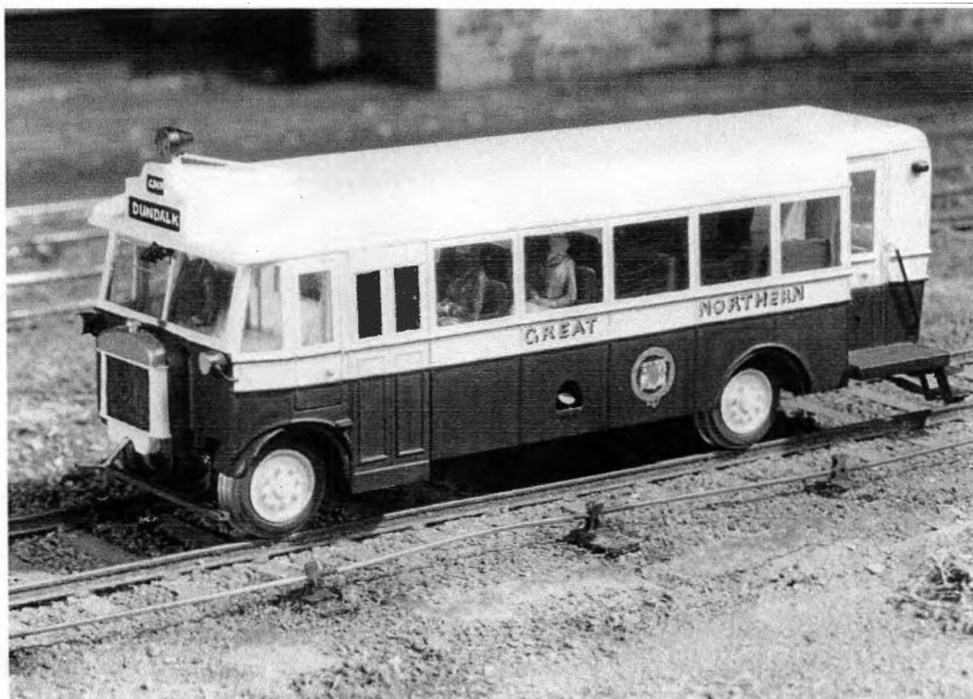
Railbus F3, built 1935. It had a patented wheel system, with flanged metal tyres outside normal pneumatic tyres.
