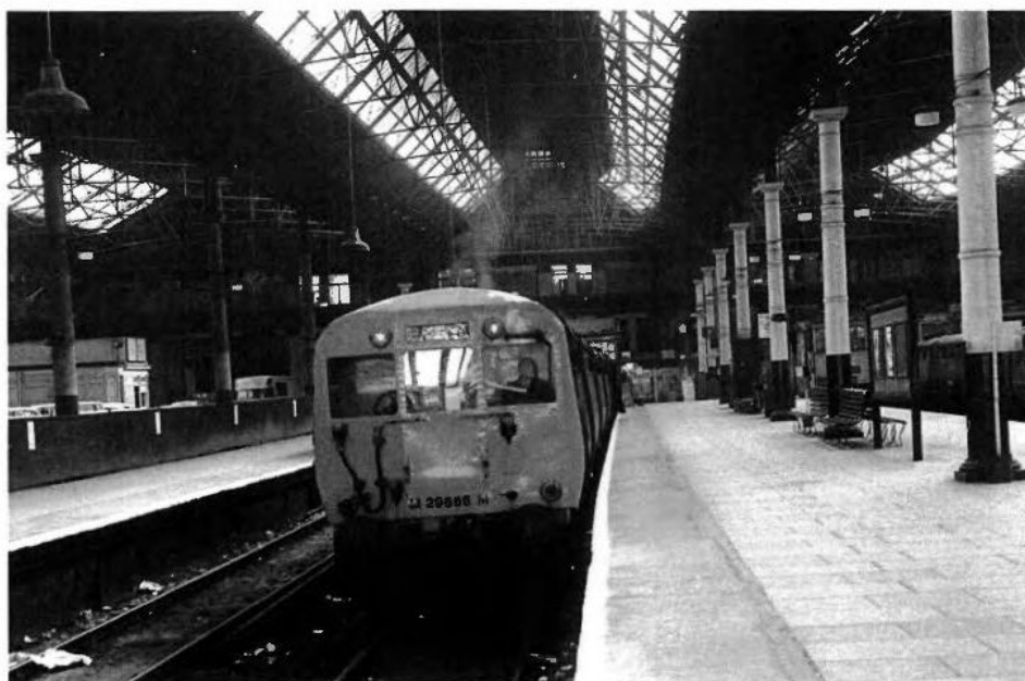
M29886M at Liverpool Exchange, photographed by John Dixon in March 1977. This is an L.M.S.-built EMU, picking up from a third rail at 630V; class was 502, introduced in 1939.
