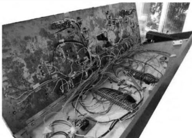
Fig.3 - Internal view of original Main Control Panel
