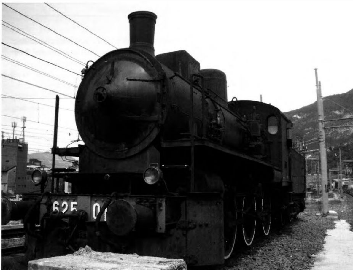
The preserved 'Tishy' in Italy, seen on a short piece of track off the north end of one of the main line platforms at Trento, on the line running north from Verona and over the Brenner Pass to Austria. The engine is a 2-6-0 with number 625 011. It has two inside cylinders but its piston valves are outside the frames and are worked by Walschaerts valve gear, also mounted outside the frames. RefSOC 1339.
