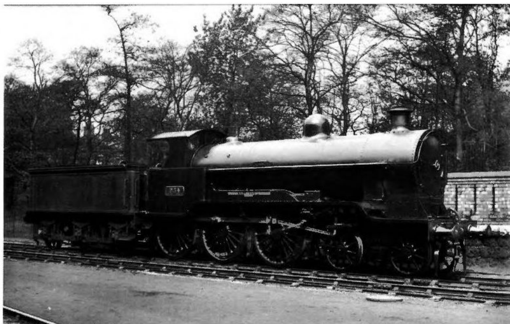
LNWR 'Tishy' No. 964 BRET HARTE, photographed at Crewe Works on 2nd May 1923, early in LMS days although the engine is in LNWR plain black livery with LNWR fittings. In the background are the gardens of the management houses. The engine has recently been rebuilt with outside Walschaerts valve gear but still with its inside piston valves and cylinders. (The reference number for the picture is CRPRT A631 (an LNWR official photograph)).
