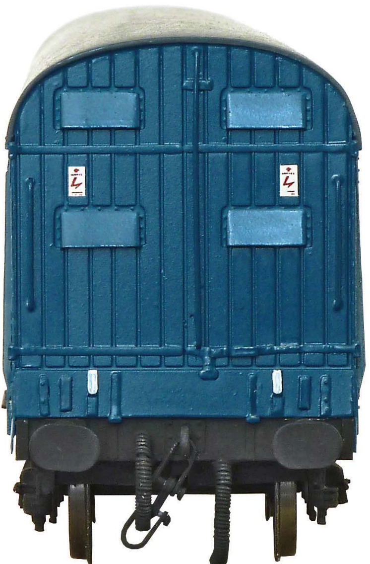
Above: This end-on view captures the challenge of making a reliable, consistent, thin roof profile from plasticard sheet. Also visible are the numerous small soldered details added to the end doors and drop-down flaps.
