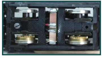
• Fit bogie side frame moulding to motor. In order to do this you will need to cut out a rectangle from the base of the plastic moulding (to allow clearance for the pick-up carrier).
