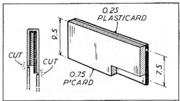
This jig does make the replication of brake safety loops much easier
